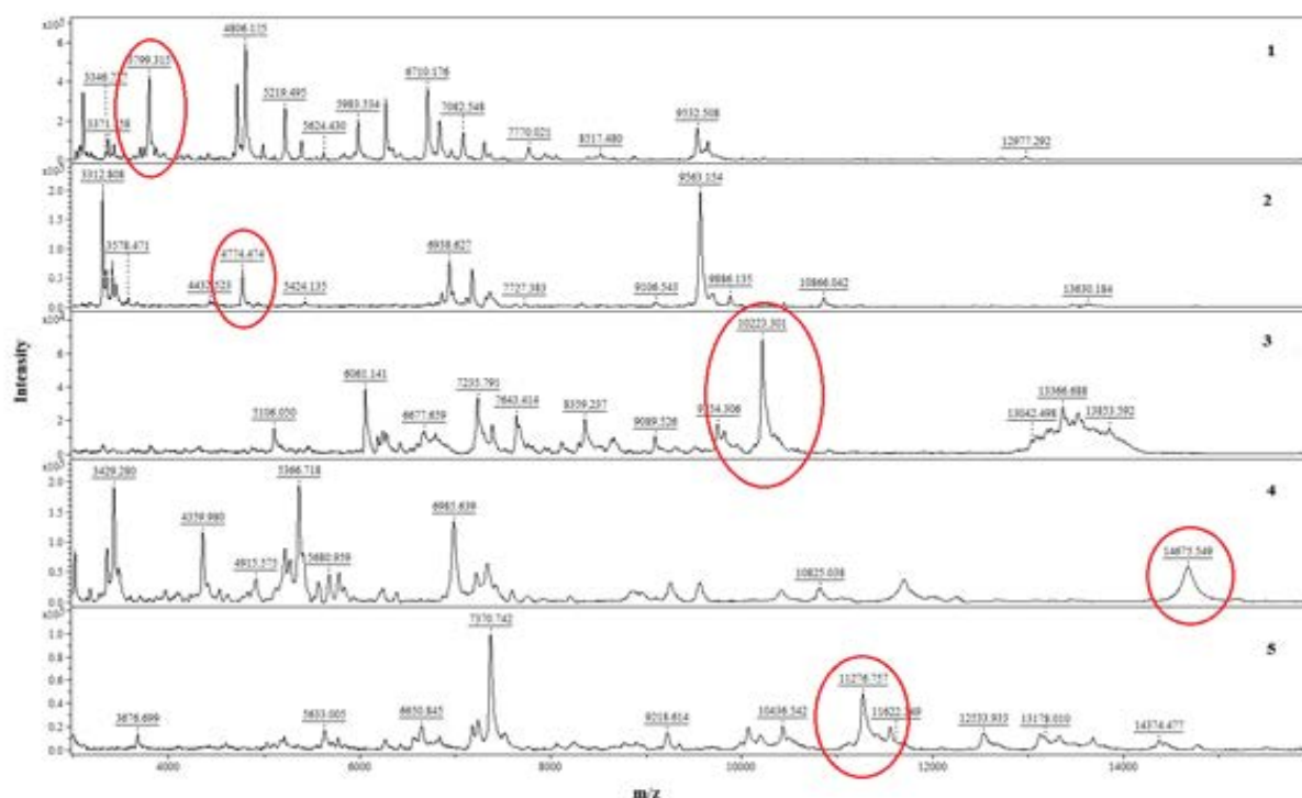
Figure 7: IC MALDI TOF MS spectra of bacteria strain. 1 - B. cereus , 2 - B. subtilis , 3 - M. luteus , 4 - S. lutea , 5 - S. aureus (1). The circle presents the unique peaks.
