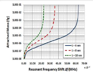
**Figure 2:** Resonant frequency shift  $\Delta f$  due to attached mass at the tip of the nanotube of cantilevered configuration of nanotube.
