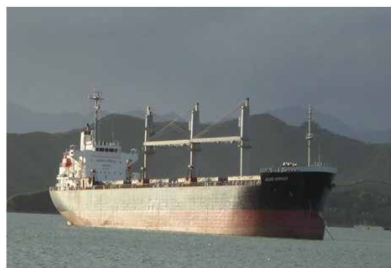
Figure 3: M/V JULES GARNIER. The ship was tested in Hiroshima, Japan in a weather condition : Cloudy and Smooth. Date test on October, 2 nd - 2002 with Main Engine type is HITACHI MAN B&W 7S35MC Mk-7 (5,180 KW×173 min -1 ), using fuel oi: Heavy Fuel oil (HFO) at each different load.
