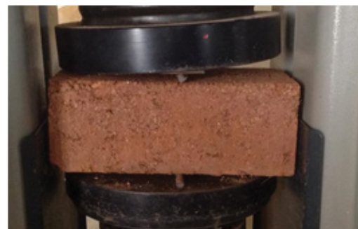
Figure 6: Set-up of tensile strength test.
