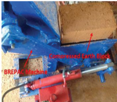
Figure 4: Pressure gauge machine for block making.
