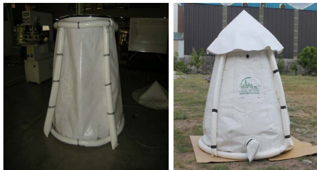
Figure 2: The 1-ton model of the collapsible silo assembled with pneumatic post and circular ring to facilitate center loading (a) and the fully-loaded unit with the top cover (b).
