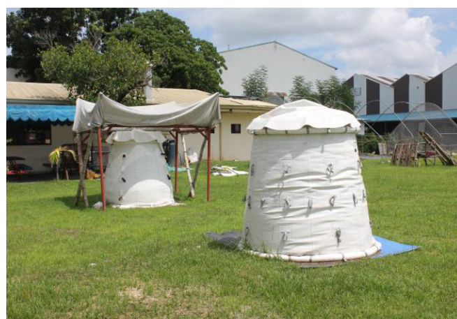
Figure 3: Outdoor experiment of the CHS model, with and without grain shed, to determine oxygen level reduction as a factor in long-term grain storage.
