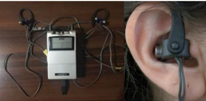
Figure 2: The Vagustim device and its in-ear shape.
