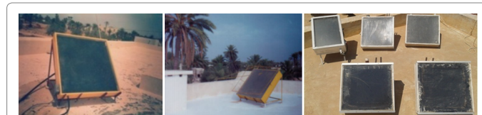
Figure 7: Integrated storage solar collector.
