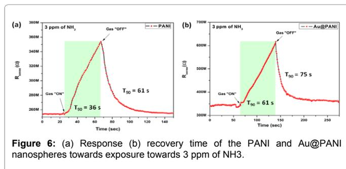
Figure 6: (a) Response (b) recovery time of the PANI and Au@PANI nanospheres towards exposure towards 3 ppm of NH<sub>3</sub>.
