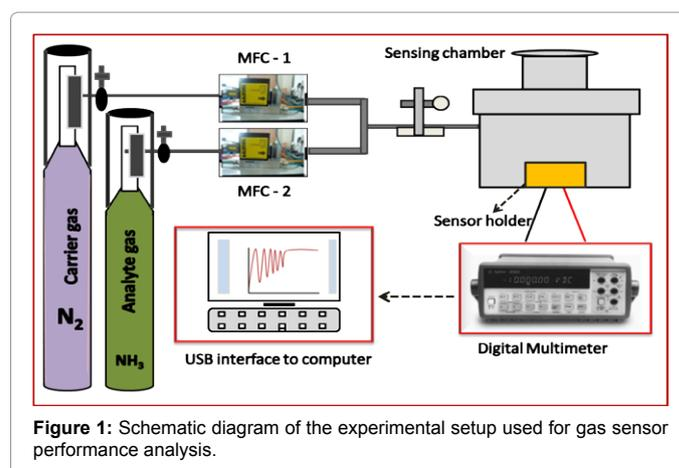
**Figure 1:** Schematic diagram of the experimental setup used for gas sensor performance analysis.
