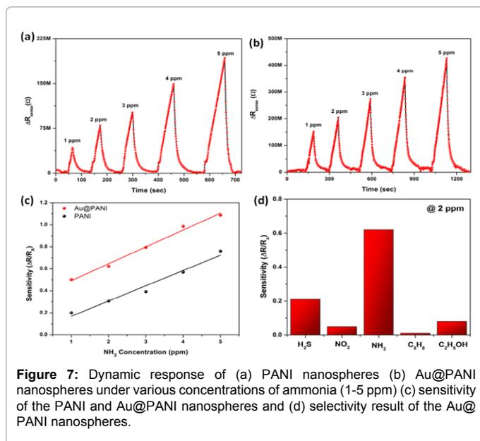
Figure 7: Dynamic response of (a) PANI nanospheres (b) Au@PANI nanospheres under various concentrations of ammonia (1-5 ppm) (c) sensitivity of the PANI and Au@PANI nanospheres and (d) selectivity result of the Au@PANI nanospheres.
