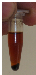
Figure 7: Close-up image of degraded crude oil and residual mineral salts at bottom.
