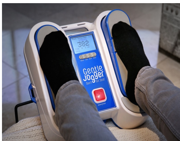
Figure 2: Gentle Jogger on bed. The Gentle Jogger is propped against a foot rail seen on the left side of the image. A retaining Velcro strap holds the Gentle Jogger in place during activation. The feet are strapped to the pedals for firm coupling (straps not shown in this image). The LED on the top displays number of steps, time and speed as walk, jog, run, and race.
