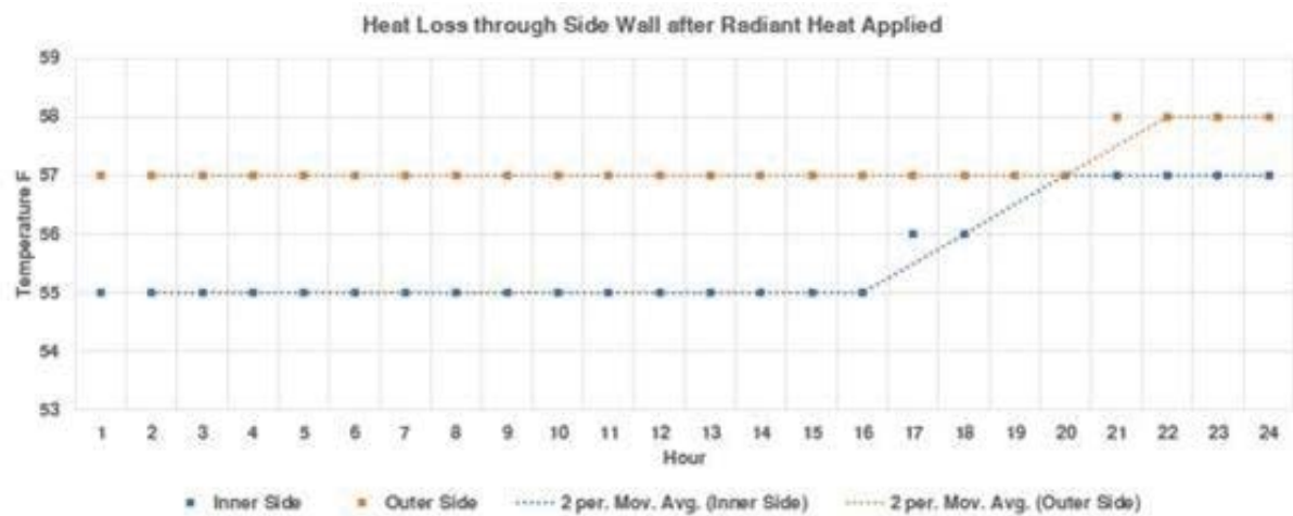
Figure 12: Heat loss through the side wall, six inches of mortar and one-inch ceramic wall.
