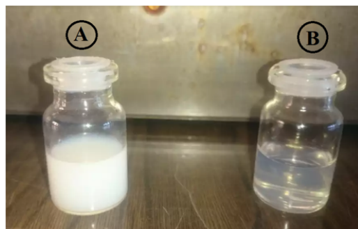
Figure 1: Nano-emulsion (O/W) of peppermint essential oil M. piperita (4%) obtained by (A) Before Sonication, (B) After Sonication.
