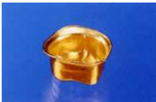
Figure 3: Gold coping made using electroforming.
