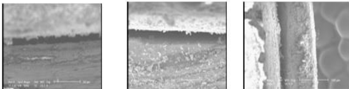
Figure 5: Electronic microscope pictures from the gap between die and electroforming restoration in shoulder type FL.
