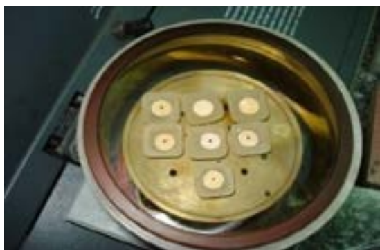
Figure 4: Plaster die mounted in brilliant acrylic and it is cutting below finish line.
