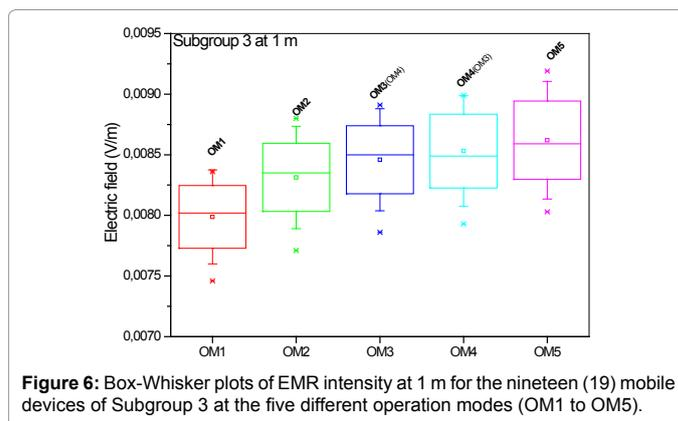
Figure 6: Box-Whisker plots of EMR intensity at 1 m for the nineteen (19) mobile devices of Subgroup 3 at the five different operation modes (OM1 to OM5).
