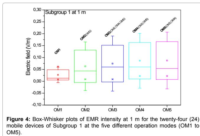
Figure 4: Box-Whisker plots of EMR intensity at 1 m for the twenty-four (24) mobile devices of Subgroup 1 at the five different operation modes (OM1 to OM5).
