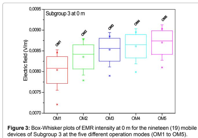
Figure 3: Box-Whisker plots of EMR intensity at 0 m for the nineteen (19) mobile devices of Subgroup 3 at the five different operation modes (OM1 to OM5).
