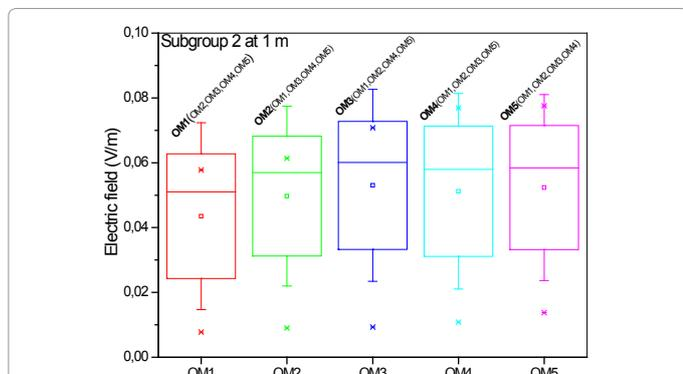
Figure 5: Box-Whisker plots of EMR intensity at 1 m for the nine (9) mobile devices of Subgroup 2 at the five different operation modes (OM1 to OM5).
