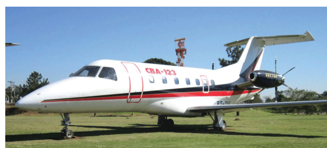
Figure 26: 19-seat CBA-123 pusher turboprop (Photo: Bento Mattos).
