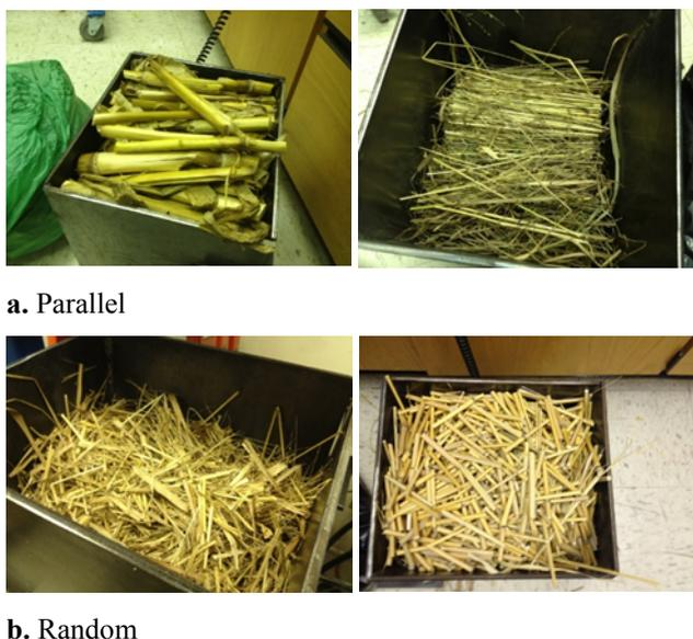
Figure 2: Arrangements/orientation of the samples.
