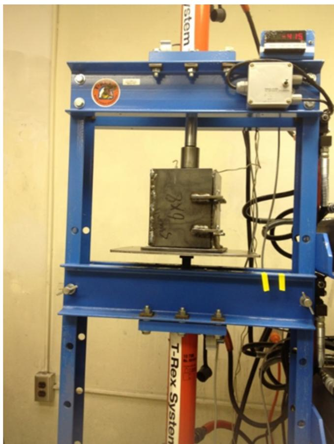
Figure 3: The T-Rex machine compressing biomass.
