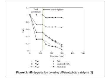
The photoreactor was irradiated by a strip composed by white light LEDs (nominal power: 6W) with wavelength emission in the range 400-800 nm or by a similar number of blue light LEDs (nominal power: 6W) with wavelength emission in the range 400-550 nm. The obtained results, reported in Figure 2, showed that only the N-doped TiO<sub>2</sub> is a photocatalyst effective under visible light.
