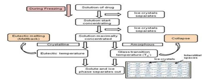
Fig. 2: Flowchart showing the concept of eutectic temperature and Tg (glass Transition) and their importance during primary drying.
