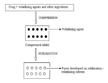
Fig. 3: Schematic Diagram of Sublimation Technique for Preparation of MDT
