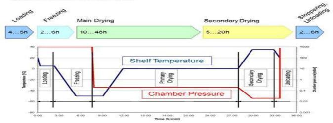
Fig. 1: Typical Freeze Drying Cycle
