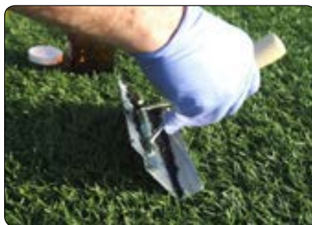
Figure 1: Example of collection methods for tire crumb rubber infill on synthetic turf fields
