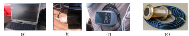
Figure 2: Hydroacoustic Instruments CruzPro fish finder PcFF-80 with a) Pc/Computer, b) Interface, c) Hand GPS, d) Transducer (Single beam echosuonder) personal documentation.
