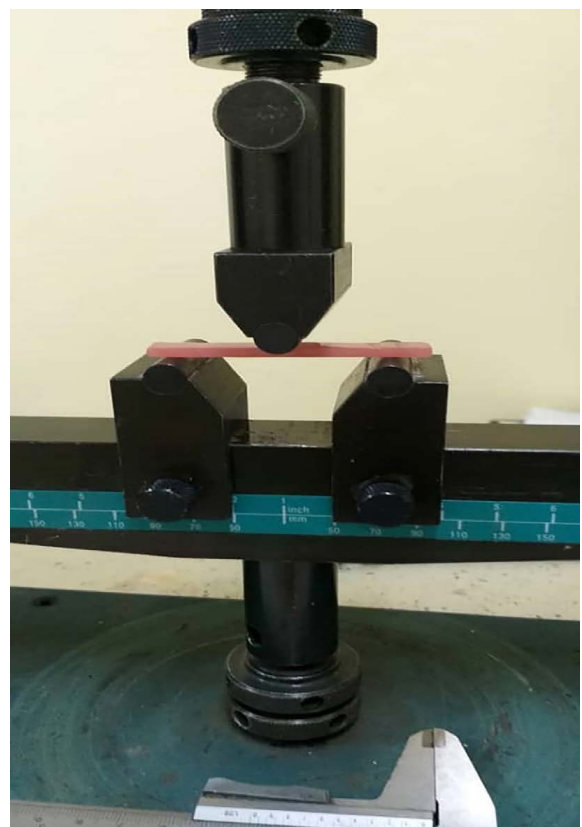
Figure 2: A 3-point bending test by the universal testing machine (DY-34 ADAMEL LHOMARGY).
