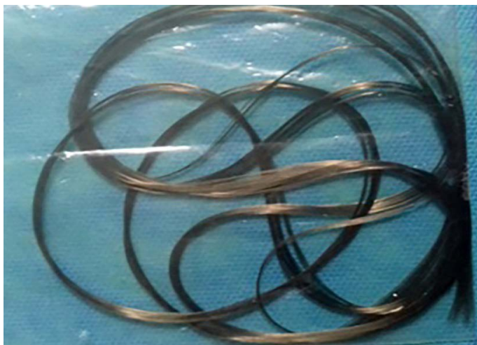
Figure 1: Basalt fibers ( 16 \pm 2 \mu\text{m} in diameter).
