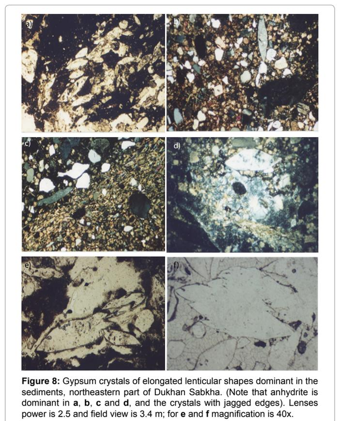
**Figure 8:** Gypsum crystals of elongated lenticular shapes dominant in the sediments, northeastern part of Dukhan Sabkha. (Note that anhydrite is dominant in a, b, c and d, and the crystals with jagged edges). Lenses power is 2.5 and field view is 3.4 m; for e and f magnification is 40x.
