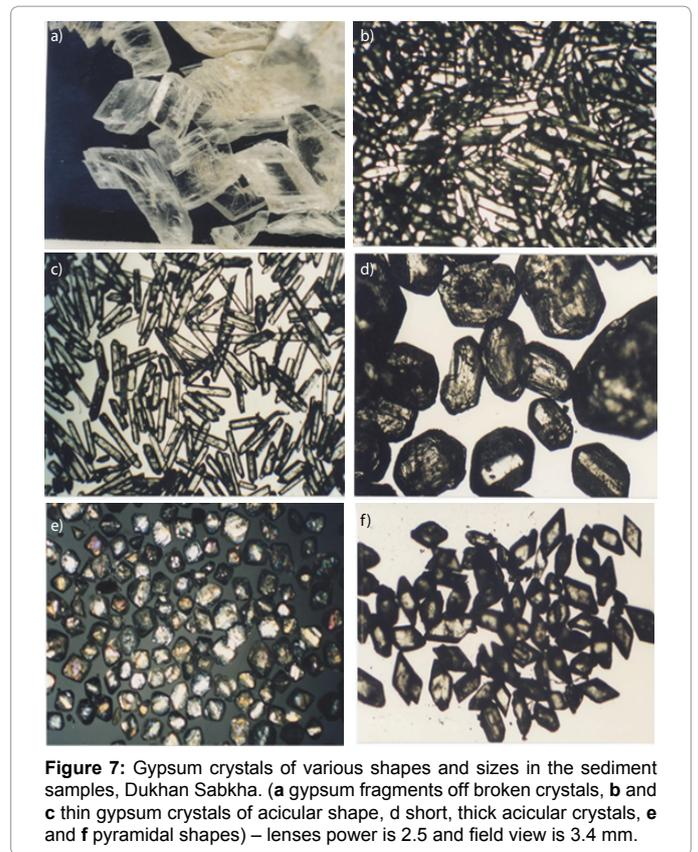
**Figure 7:** Gypsum crystals of various shapes and sizes in the sediment samples, Dukhan Sabkha. (a gypsum fragments off broken crystals, b and c thin gypsum crystals of acicular shape, d short, thick acicular crystals, e and f pyramidal shapes) – lenses power is 2.5 and field view is 3.4 mm.
