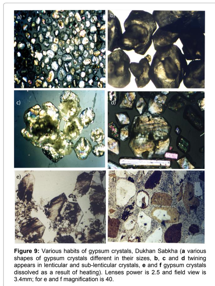
**Figure 9:** Various habits of gypsum crystals, Dukhan Sabkha (a various shapes of gypsum crystals different in their sizes, b, c and d twinning appears in lenticular and sub-lenticular crystals, e and f gypsum crystals dissolved as a result of heating). Lenses power is 2.5 and field view is 3.4mm; for e and f magnification is 40.
