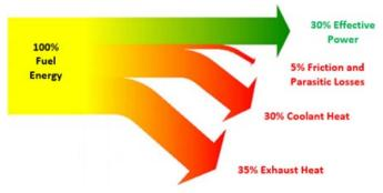
Figure 16: Gasoline engine efficiency diagram ("Triple A" image).
