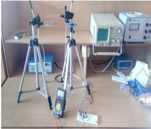
Figure 11: RF harvesting system with 8-stage multiplier circuit.
