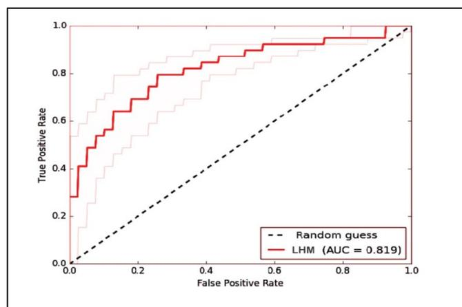
Figure 9: AUC graph shows the Landslide Hazard Map Validation up to 81.9%.
