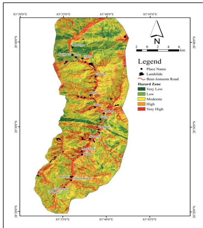
Figure 6: Landslide Hazard Map Calculated by Weight of Evidence Method.
