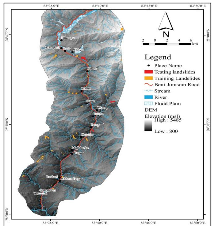
Figure 4: Landslide inventory map of study area.
