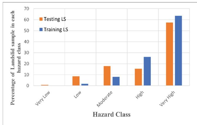
Figure 8: Landslide Distribution in Different Hazard Zone Using the Training Data Sets and Validating Data Sets.
