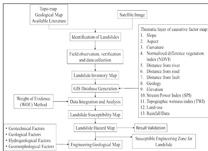
Figure 2: Methodology Flow Chart of Landslide Hazard Analysis by Weight of Evidence Method
