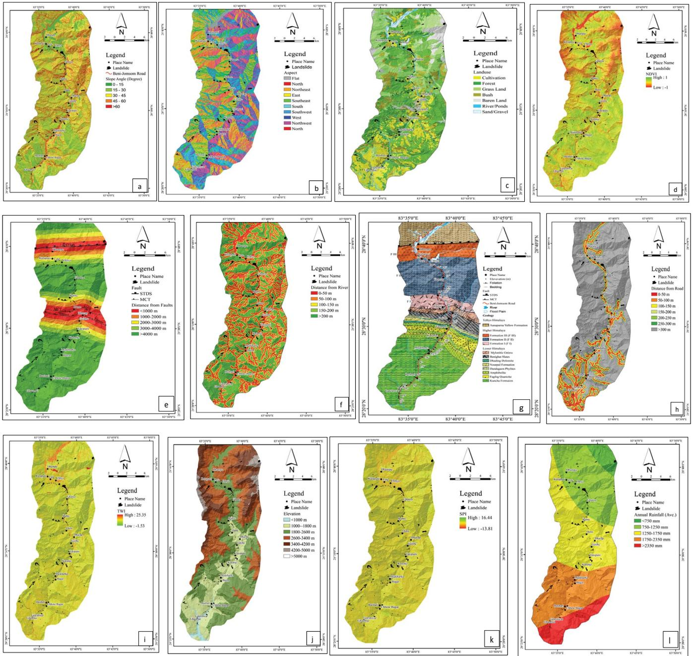
Figure 5: a. slope map, b. Aspect map, c. landuse map, d. normalized difference vegetation index, e. distance from fault, f. distance from river, g. geology, h. distance from road, i. Topographic wetness index map, j. elevation map, k. stream power index, l. average rainfall map.
