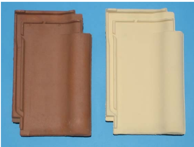
Figure 15: Crude red-brick ( \beta_s=0.53 ) and painted one (bright brown, \beta_s=0.30 ).
