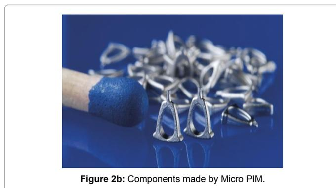
Figure 2b: Components made by Micro PIM.
