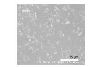
Figure 1: ESEM of glaze with 10wt. % zircon.
