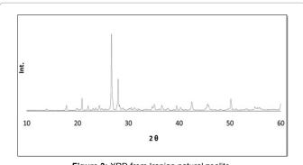
Figure 3: XRD from Iranian natural zeolite.
