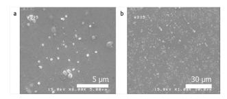
**Figure 5:** FESEM of standard frit containing 3 wt.%  $TiO_2$  and 7 wt.% zeolite; a) morphology of crystal in the range of 25-500 nm, and 85 nm on average, b) fine distribution of crystals.
