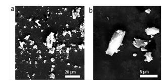
Figure 2: FESEM of standard frit with a) 5, and b) 10wt. % titania.
