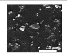
Figure 6: FESEM of standard frit containing 3 wt.%  $\rm TiO_2$  and 7 wt.% kaolin.
