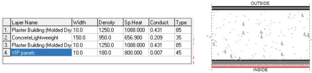
Figure 26: Roof slab section.
