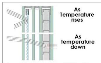
Figure 9 Glass incorporated salt hydrate serves as PCM's
