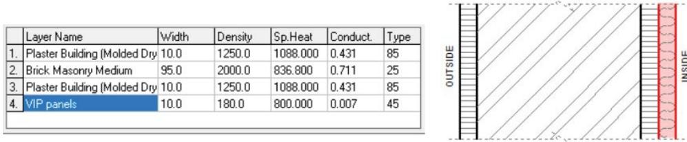
Figure 25: Wall section.
