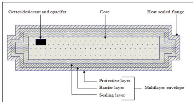
Fig.4. Schematic of a VIP
