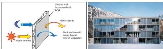
Figure 12 Use of paraffin wax & Bee wax as PCM's in concrete
