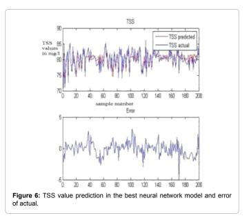
effluent treatment plant of dairy industry. It is concluded that, ANN provides an effective analysing and diagnosing tool to understand and simulate the non-linear behaviour of the plant.
