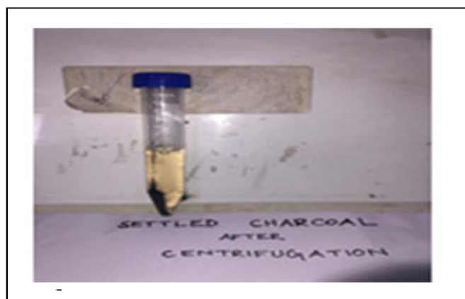
Figure 2: Human serum sample with settled charcoal after centrifugation for 40 minutes.
