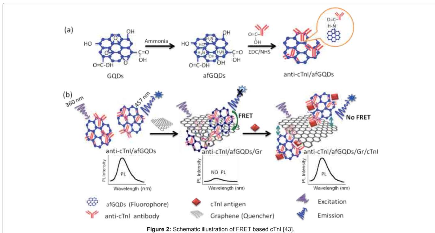
Figure 2: Schematic illustration of FRET based cTnI [43].
