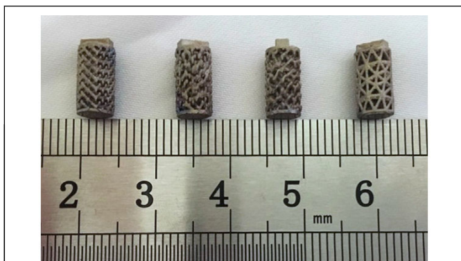
Figure 1B iv: 3D printed porous titanium scaffolds with different pore structures. Reproduced from Wang, H. et al. The effect of 3D- printed Ti(6)Al(4)V scaffolds with various macropore structures on osteointegration and osteogenesis: A biomechanical evaluation. J Mech Behav Biomed Mater. (2018). https://doi.org/10.1016/j.jmbbm.2018.08.049
