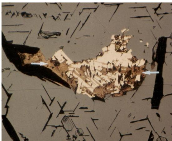
**Figure 15:** Chalcopyrite replaced by valleriite in magnetite which contains brucite-lamellae arranged along [111]-magnetite. Reflected light, oil immersion objective, longer edge 450  $\mu$ . – Gole Gohar/Iran
