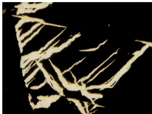
**Figure 4:** Identical with A/3. Note the luminous appearance of mackinawite which occurs in the bright 45°-degree position. Reflected light, crossed polars, oil immersion objective, longer edge 450 μ. – Outokumpu/Finland
