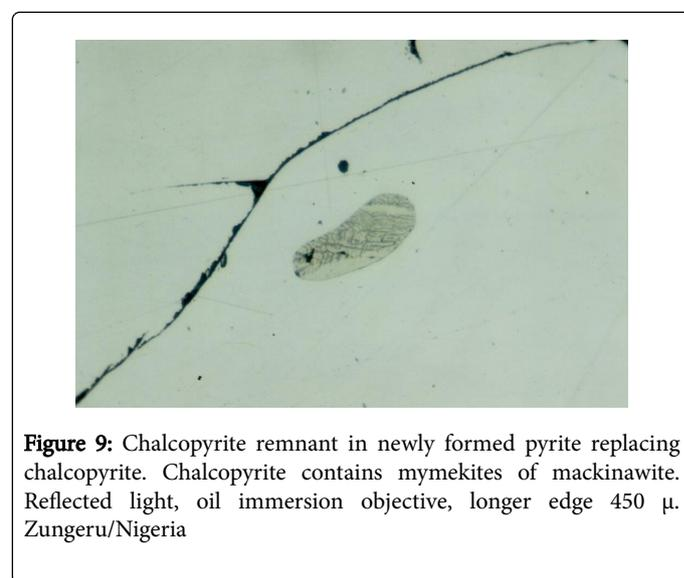
**Figure 9:** Chalcopyrite remnant in newly formed pyrite replacing chalcopyrite. Chalcopyrite contains mymekites of mackinawite. Reflected light, oil immersion objective, longer edge 450  $\mu$ . Zungeru/Nigeria
