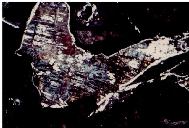
**Figure 16:** Metamorphically decomposed valleriite in a silicate groundmass (black). Spot-like distributed and concentrated along the rim of the original valleriite crystal, magnetite occurs (brightest mineral). Reflected light, oil immersion objective, longer edge 450  $\mu$ . – Outokumpu/Finland
