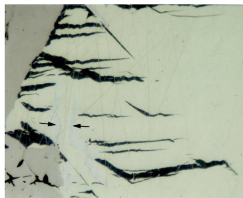
**Figure 3:** Pyrrhotite (brownish) and chalcopyrite (yellow and slightly brighter than pyrrhotite). The latter contains flame-like inclusions of mackinawite mostly in the dark cutting position. The brightest cutting position is arrowed. Reflected light, oil immersion objective, longer edge 450 μ. – Outokumpu/Finland
