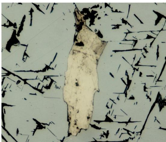
**Figure 14:** Valleriite in the bright cutting position included in magnetite which contains oriented arranged (parallel to [111]-magnetite) brucite-lamellae. Reflected light, oil immersion objective, longer edge 450  $\mu$ . – Gole Gohar/Iran
