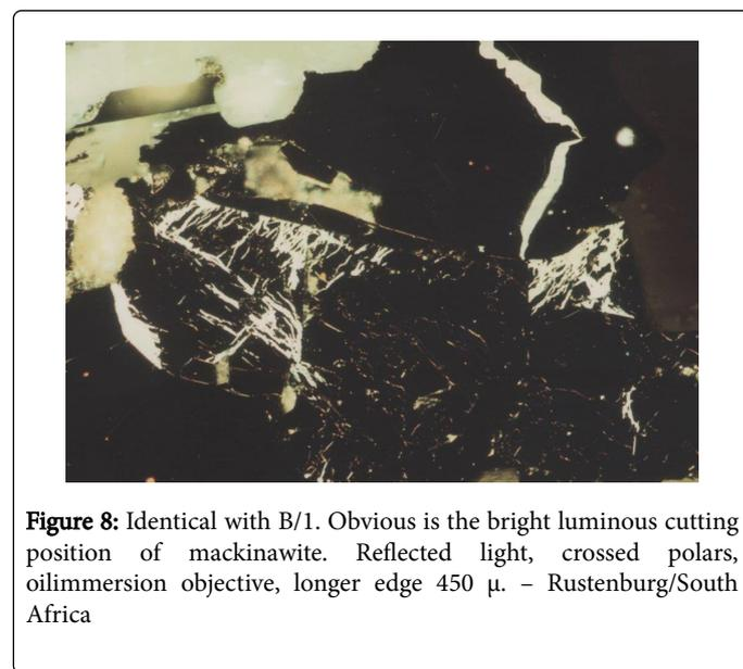
**Figure 8:** Identical with B/1. Obvious is the bright luminous cutting position of mackinawite. Reflected light, crossed polars, oilimmersion objective, longer edge 450  $\mu$ . – Rustenburg/South Africa
