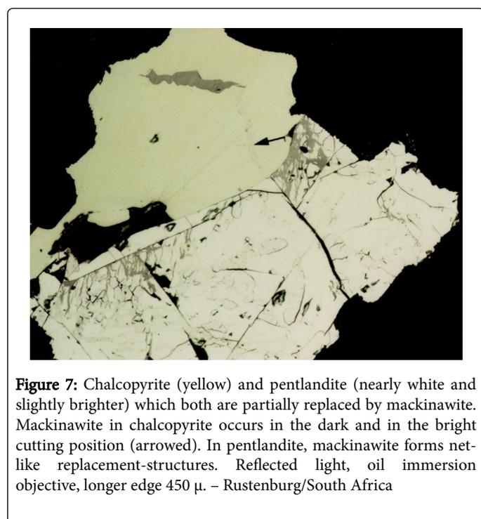
**Figure 7:** Chalcopyrite (yellow) and pentlandite (nearly white and slightly brighter) which both are partially replaced by mackinawite. Mackinawite in chalcopyrite occurs in the dark and in the bright cutting position (arrowed). In pentlandite, mackinawite forms net-like replacement-structures. Reflected light, oil immersion objective, longer edge 450  $\mu$ . – Rustenburg/South Africa
