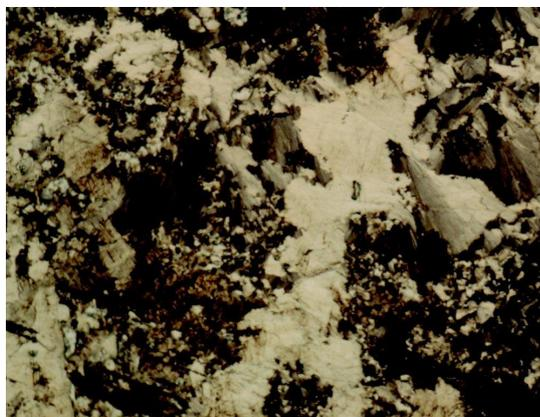
**Figure 10:** Aggregate consisting of mostly radiating arranged valleriite crystals. Reflected light, oil immersion objective, longer edge 450  $\mu$ . – Palabora/South Africa
