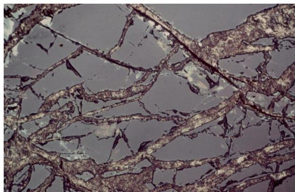
**Figure 13:** Valleriite occurring along cracks and fissures of magnetite (grey). Reflected light, oil immersion objective, longer edge 450  $\mu$ . – Domokos/Greece
