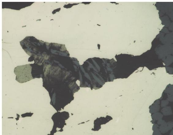
**Figure 12:** Valleriite in various cutting positions (brown to black) intimately intergrown with lensoidal-shaped magnetite (grey) embedded in pyrrhotite. Reflected light, oil immersion objective, longer edge 450  $\mu$ . – Domokos/Greece
