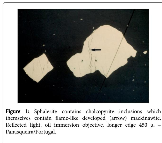
**Figure 1:** Sphalerite contains chalcopyrite inclusions which themselves contain flame-like developed (arrow) mackinawite. Reflected light, oil immersion objective, longer edge 450 μ. – Panasqueira/Portugal.
