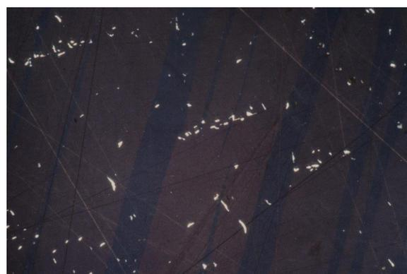
**Figure 6:** Tiny mackinawite crystals arranged in the form of strings of pearls in chalcopyrite. Note the twinning of the host chalcopyrite and the fact that all the mackinawite crystals reveal the same brightness and therefore the same cutting position. Reflected light, oil immersion objective, longer edge 450  $\mu$ . - Broken Hill/Australia
