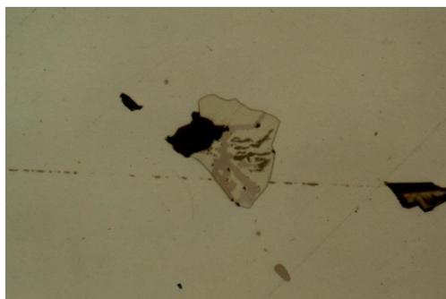
**Figure 5:** Remnants of chalcopyrite (yellow) and pyrrhotite (brownish) in pyrite formed by pyritization of the first two minerals. Chalcopyrite contains newly-formed myrmekites of mackinawite (dark-grey). Quartz is black. Reflected light, oil immersion objective, longer edge 450  $\mu$ . - Hagendorf-South/Germany
