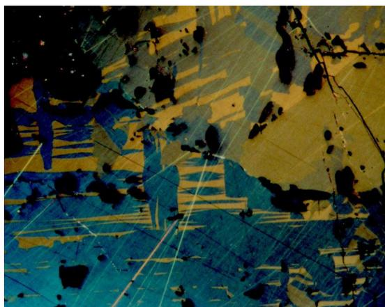
**Figure 17:** Chalcopyrite with polysynthetic arranged oleander leaf-like twins. The blue colour tint is attributed to the used objective which has a metal improved surface. Reflected light, oil immersion objective, crossed polars, longer edge 450  $\mu$ . – Hagendorf-South/Germany
