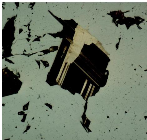
**Figure 11:** Parquet-like, polysynthetic twinning of valleriite caused by translation. The crystal which is embedded in magnetite shows a cutting position in which the brightest and lowest reflecting positions occur together. Reflected light, oil immersion objective, longer edge 450  $\mu$ . – Palabora
