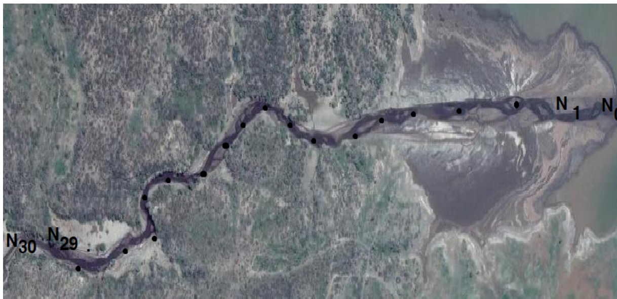
Figure 1: Symbolized river nodes and reaches schematization.
