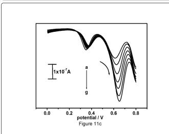
**Figure 11c:** Differential pulse voltammograms of (a) 4  $\mu$ M, (b) 8  $\mu$ M, (c) 12  $\mu$ M, (d) 16  $\mu$ M, (e) 20  $\mu$ M, (f) 24  $\mu$ M (g) 28  $\mu$ M FA in 0.2 M phosphate buffer solution of pH 7.2 in presence of 6  $\mu$ M PA at Pregabalin modified carbon paste electrode.
