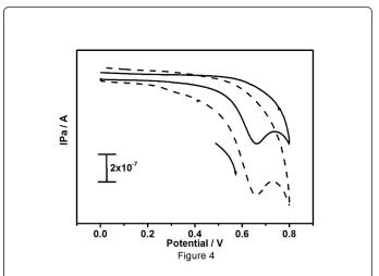
**Figure 4:** Cyclic voltammograms of 10  $\mu$ M FA in 0.2 M phosphate buffer solution of pH 7.2 at BCPE (solid lines) and Pregabalin MCPE (dashed line) with scan rate of 30 mV/s.
