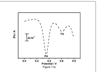
**Figure 11a:** Differential pulse voltammogram of mixture solution of paracetamol (12  $\mu$ M), folic acid (4  $\mu$ M) in 0.2 M phosphate buffer solution of pH 7.2 at pregabalin modified carbon paste electrode.
