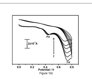
**Figure 10c:** Cyclic voltammograms for simultaneous determination of (a) 10  $\mu$ M, (b) 20  $\mu$ M, (c) 30  $\mu$ M, (d) 40  $\mu$ M, (e) 50  $\mu$ M (f) 60  $\mu$ M FA in 0.2 M phosphate buffer solution of pH 7.2 in presence of 15  $\mu$ M PA at Pregabalin modified carbon paste electrode with scan rate of 30 mV/s.
