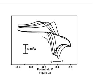
**Figure 9a:** Cyclic voltammograms of 10  $\mu$ M PA in different pH (a-d: 6 to 7.5) at pregabalin modified carbon paste electrode with a scan rate of 30 mV/s.
