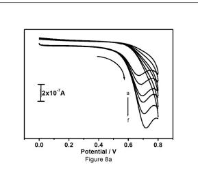
**Figure 8a:** Cyclic voltammograms for different concentration of FA (a-f; 10  $\mu$ M-60  $\mu$ M) at pregabalin modified carbon paste electrode with scan rate of 30 mV/s.
