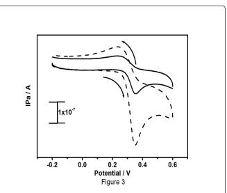
**Figure 3:** Cyclic voltammograms of 10  $\mu$ M PA in 0.2 M phosphate buffer solution of pH 7.2 at BCPE (solid line) and Pregabalin MCPE (dashed line) with scan rate of 30 mV/s.
