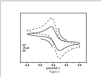
**Figure 2:** Cyclic voltammograms of 1 mM potassium ferrocyanide at BCPE (solid line), Pregabalin MCPE (dashed line) in 1M KCl scan rate of 100 mV/s.
