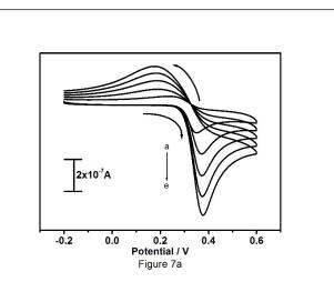
**Figure 7a:** Cyclic voltammograms for different concentration of PA (a-e; 10  $\mu$ M-50  $\mu$ M) at pregabalin modified carbon paste electrode with scan rate of 30 mV/s.
