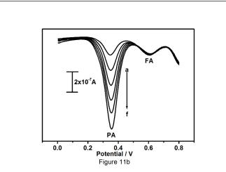
**Figure 11b:** Differential pulse voltammograms of (a) 4  $\mu$ M, (b) 8  $\mu$ M, (c) 12  $\mu$ M, (d) 16  $\mu$ M, (e) 20  $\mu$ M, (f) 24  $\mu$ M PA in 0.2 M phosphate buffer solution of pH 7.2 in presence of 6  $\mu$ M FA at Pregabalin modified carbon paste electrode.
