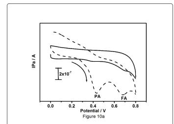
**Figure 10a:** Cyclic voltammograms for mixture solution of paracetamol (10  $\mu$ M) and folic acid (12  $\mu$ M) in 0.2 M phosphate buffer solution of pH 7.2 at BCPE (solid line), pregabalin modified carbon paste electrode (dashed line) with scan rate of 30 mV/s.
