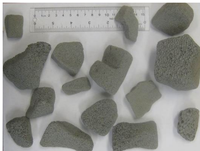
Figure 7: Chunks of glass foam for insulation under roads.
