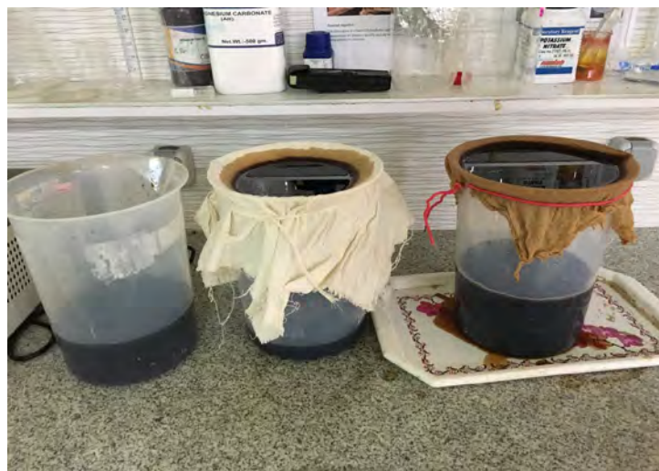
Figure 6: The samples were filtered so as to separate solid and liquid parts.
