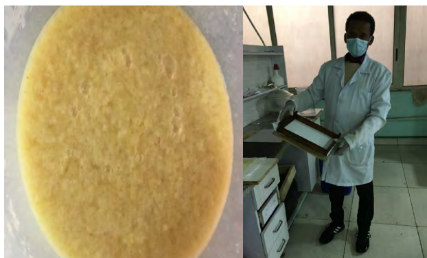
Figure 10: Fabricated Mold Casting of Paper and produced pulp.
