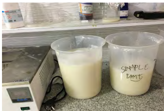
Figure 9: Pulp produced after digestions and bleaching.
