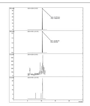
**Figure 2:** Selected MRM chromatograms for 6-monoacetylmorphine (6-MAM), in which it is evident the ion suppression due to the matrix effect.
