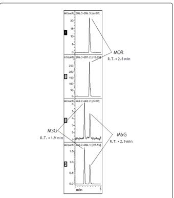
Figure 1: Selected MRM chromatograms of morphine (MOR), morphine-3-β-D-glucuronide (M3G) and morphine-6-β-Dglucuronide (M6G) (R.T.=Retention Time).
