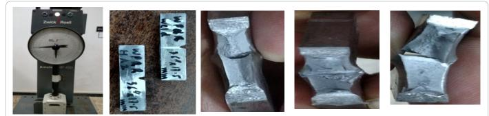
Figure 3: (Sequence of Picture Left to right): Charpy Impact test machine, CVN weld and HAZ test specimen, fractured appearance of coil CVN specimen, Fractured surface of CVN weld specimen, Fractured surface of HAZ specimen.
