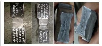
**Figure 1:** (Sequence of Picture Left to right): Prepared marked tensile specimen, fractured tensile specimen, fractured tensile specimen cone appearance, fractured tensile specimen cup appearance.
