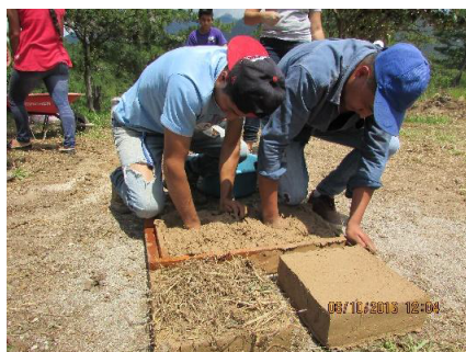
Figure 14: Training of workers making adobe blocks (FUNDASAL).
