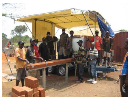
Figure 9: Oskam's mobile compresses earth block machine working in Africa.
