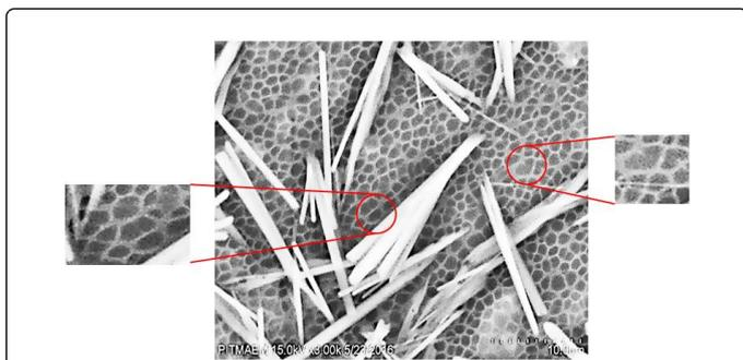
**Figure 5:** SEM micrographs of CS/AM/GO hydrogels, A Indicates drug beads loaded hydrogel at 1000X magnification, Hole defect of graphene oxide is also indicated.
