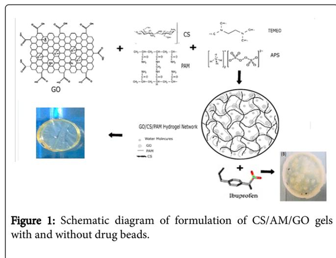
Figure 1: Schematic diagram of formulation of CS/AM/GO gels with and without drug beads.
