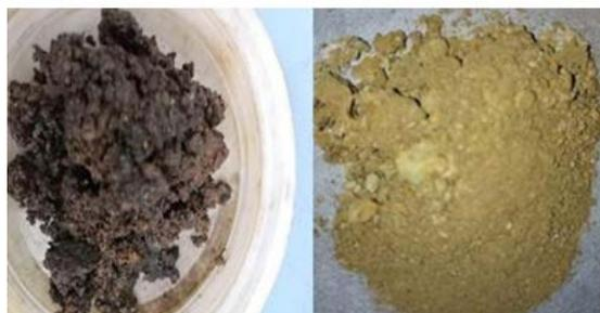
Figure 3: Left to right: The plugging sample and its inorganic part.
