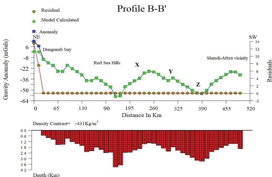
Figure 9: Gravity Anomaly and 2D density-depth crustal-mantle model along Profile B-B'.
