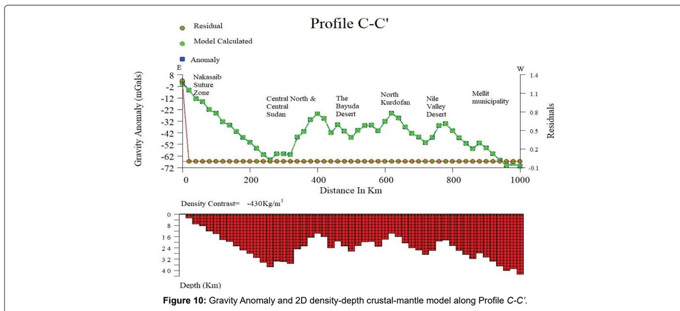
Figure 10: Gravity Anomaly and 2D density-depth crustal-mantle model along Profile C-C'.
