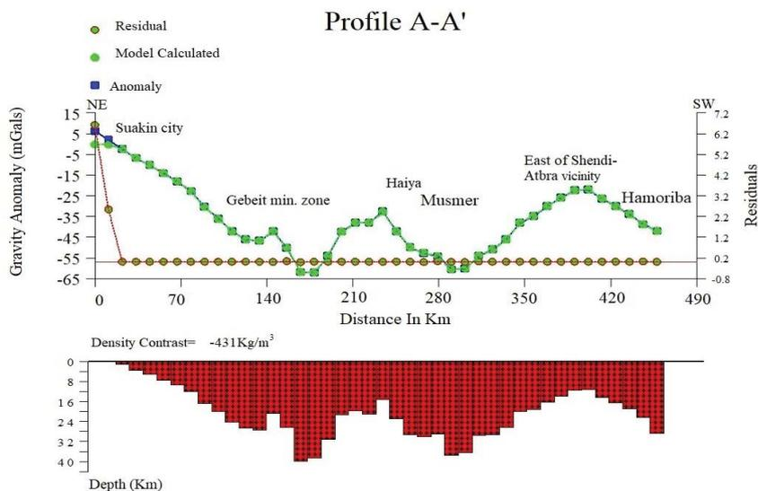
Figure 8: Gravity Anomaly and 2D density-depth crustal-mantle model along Profile A-A'.
