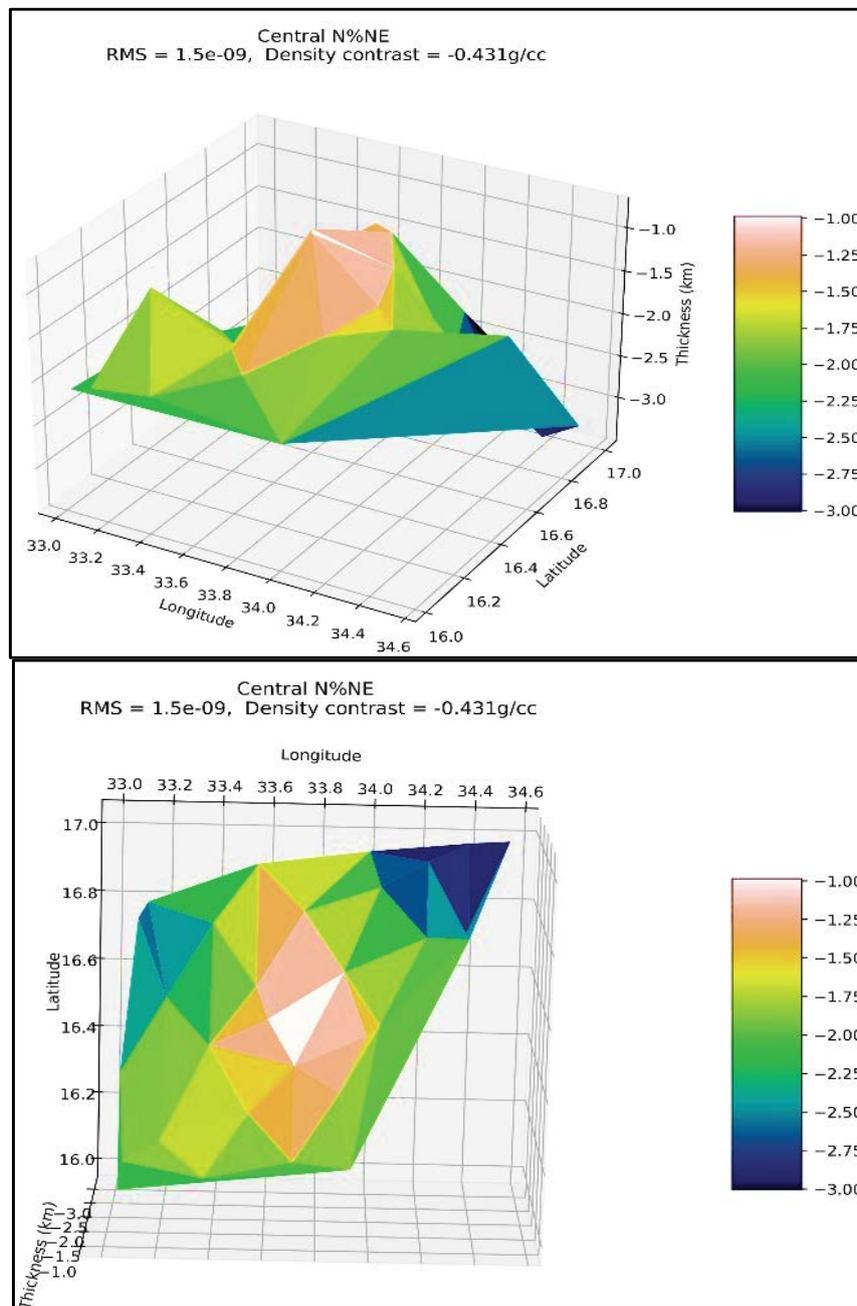
Figure 11: 3D inverted model generated from the 3D gravity anomaly inversion as looked from Above (left-side figure) and NW direction (right-side figure).
