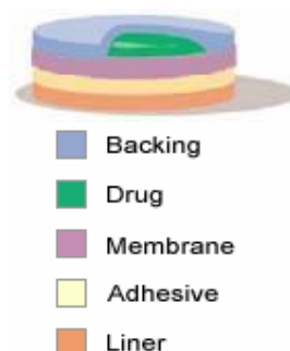
Fig.4. Drug reservoir in adhesive patch and its different component 12,15
