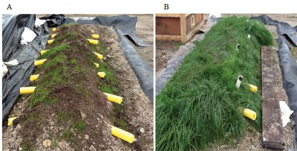
Figure 2: (A) Ecopiles two weeks after construction in June 2013 (day 14) (B) Ecopiles two months after construction in August 2013 (day 56).
