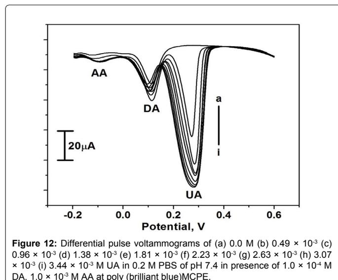
**Figure 12:** Differential pulse voltammograms of (a) 0.0 M (b)  $0.49 \times 10^{-3}$  (c)  $0.96 \times 10^{-3}$  (d)  $1.38 \times 10^{-3}$  (e)  $1.81 \times 10^{-3}$  (f)  $2.23 \times 10^{-3}$  (g)  $2.63 \times 10^{-3}$  (h)  $3.07 \times 10^{-3}$  (i)  $3.44 \times 10^{-3}$  M UA in 0.2 M PBS of pH 7.4 in presence of  $1.0 \times 10^{-4}$  M DA,  $1.0 \times 10^{-3}$  M AA at poly (brilliant blue)MCPE.
