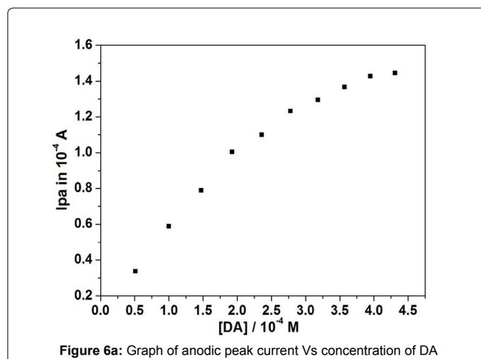
**Figure 6a:** Graph of anodic peak current Vs concentration of DA
