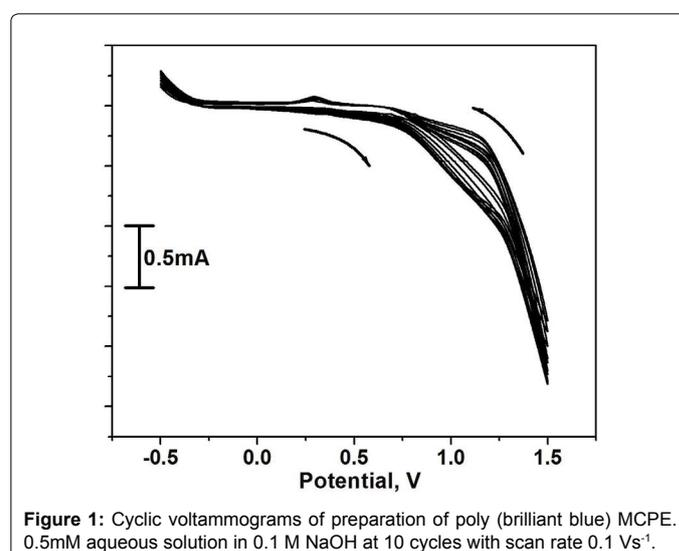
Figure 1: Cyclic voltammograms of preparation of poly (brilliant blue) MCPE. 0.5mM aqueous solution in 0.1 M NaOH at 10 cycles with scan rate 0.1 Vs<sup>-1</sup>.
