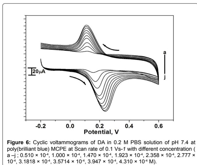
**Figure 6:** Cyclic voltammograms of DA in 0.2 M PBS solution of pH 7.4 at poly(brilliant blue) MCPE at Scan rate of 0.1 Vs<sup>-1</sup> with different concentration ( a-j ;  $0.510 \times 10^{-4}$ ,  $1.000 \times 10^{-4}$ ,  $1.470 \times 10^{-4}$ ,  $1.923 \times 10^{-4}$ ,  $2.358 \times 10^{-4}$ ,  $2.777 \times 10^{-4}$ ,  $3.1818 \times 10^{-4}$ ,  $3.5714 \times 10^{-4}$ ,  $3.947 \times 10^{-4}$ ,  $4.310 \times 10^{-4}$  M).
