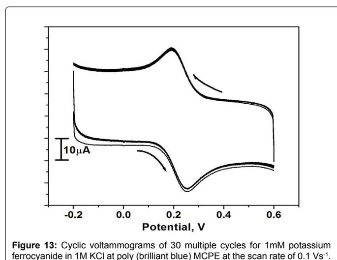
**Figure 13:** Cyclic voltammograms of 30 multiple cycles for 1mM potassium ferrocyanide in 1M KCl at poly (brilliant blue) MCPE at the scan rate of 0.1 Vs<sup>-1</sup>.
