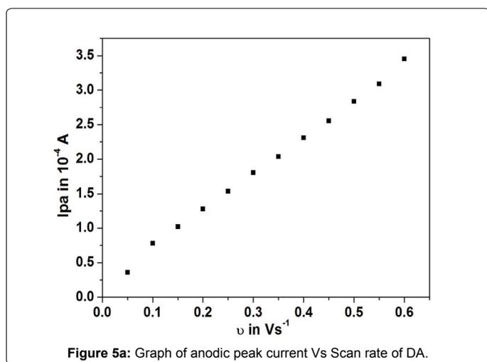
**Figure 5a:** Graph of anodic peak current Vs Scan rate of DA.
