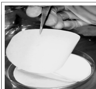
Figure 3: PVC filter membrane collected from the drum collector.
