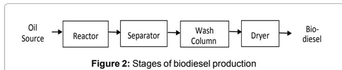
Figure 2: Stages of biodiesel production
