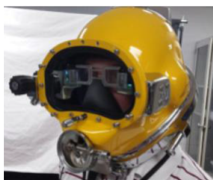
Figure 9: A new AR helmet Designed by US navy for underwater missions.
